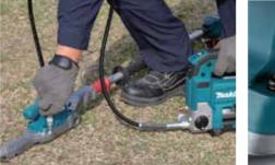
Users who do not own a grease gun can remove the bolt and supply grease with a grease tube as with our current models.
