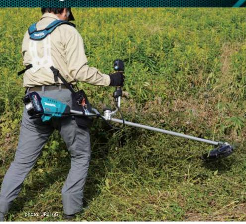
Multi functional control panel: near right hand position for easy access and operation
