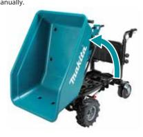
• The electric dump is limited to use on a flat ground, therefore, the machine is equipped with a level gauge to check the leveling of the machine.
