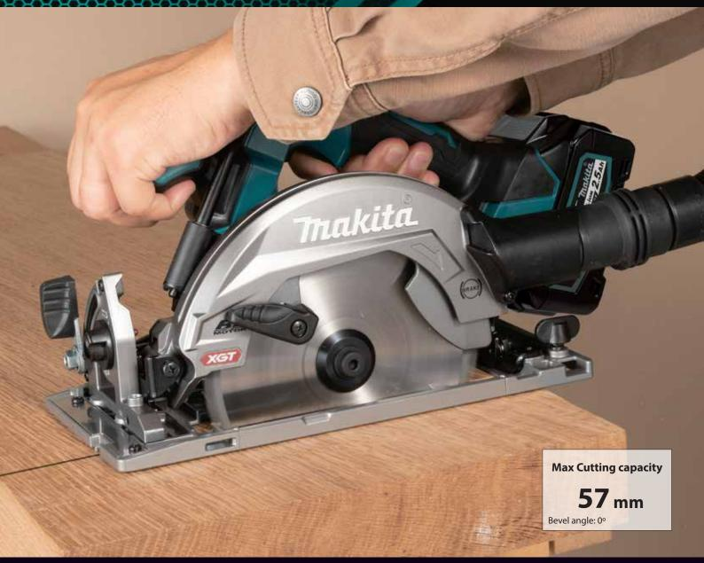
Work amount on a full battery charge BL4025 approx **110** cuts. Test material: 50mm x 300mm Melapi
