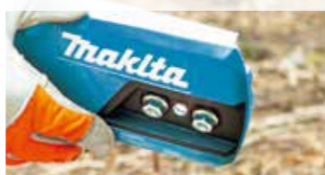
Captive nuts prevent loss of nut when removing a sprocket cover to replace a guide bar or a saw chain.
