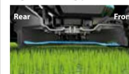
The blade is designed so that it tilts towards the front side of the mower when attached, preventing double-cutting for reduced current consumption.
