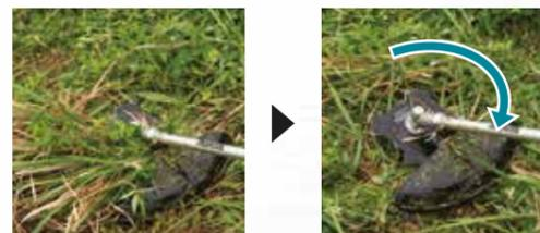
Reverse switch for clearing entangled weeds and grass from cutting head
