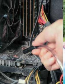
Flexible nozzle complete set Part No. 191X21-8 For blowing dust away from OA
