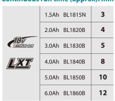
On a single full battery charge with max air setting
