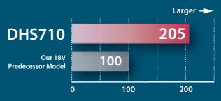
Note: 1. The test results depend to a great extent on the hardness of materials, etc. 2. The numbers in the charts are relative values when the capacities of Makita BSS611 are indexed at 100. Power source: DHS710 by two 18V-3.0Ah BL1830 Blade used for tests: Saw blade supplied with each model
